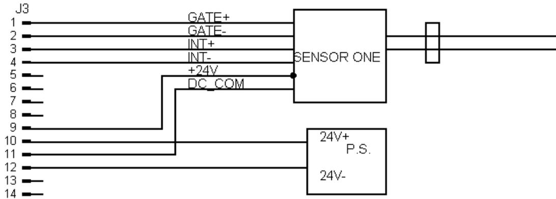
Connections for one 24V SSI transducer
