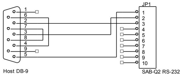
Figure 2: Diagram of SAB-Q2 RS-232 Serial Cable
