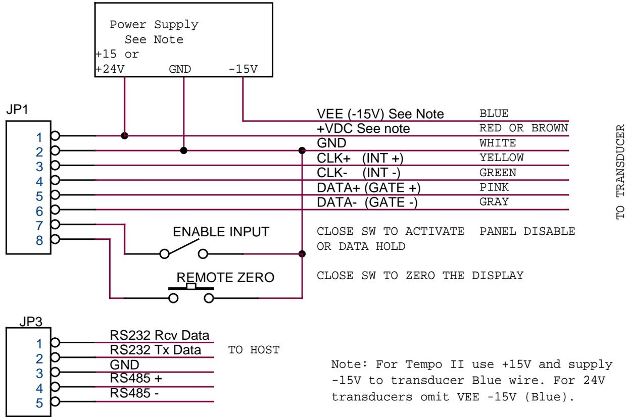
Figure 1: TDD Connections
