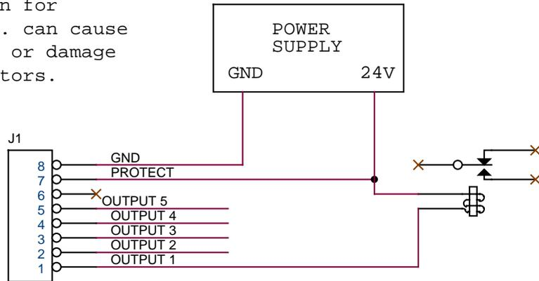
If you use the TDD internal kickback protection you must connect the + Power supply to J1 Pin 7 of the TDD.
