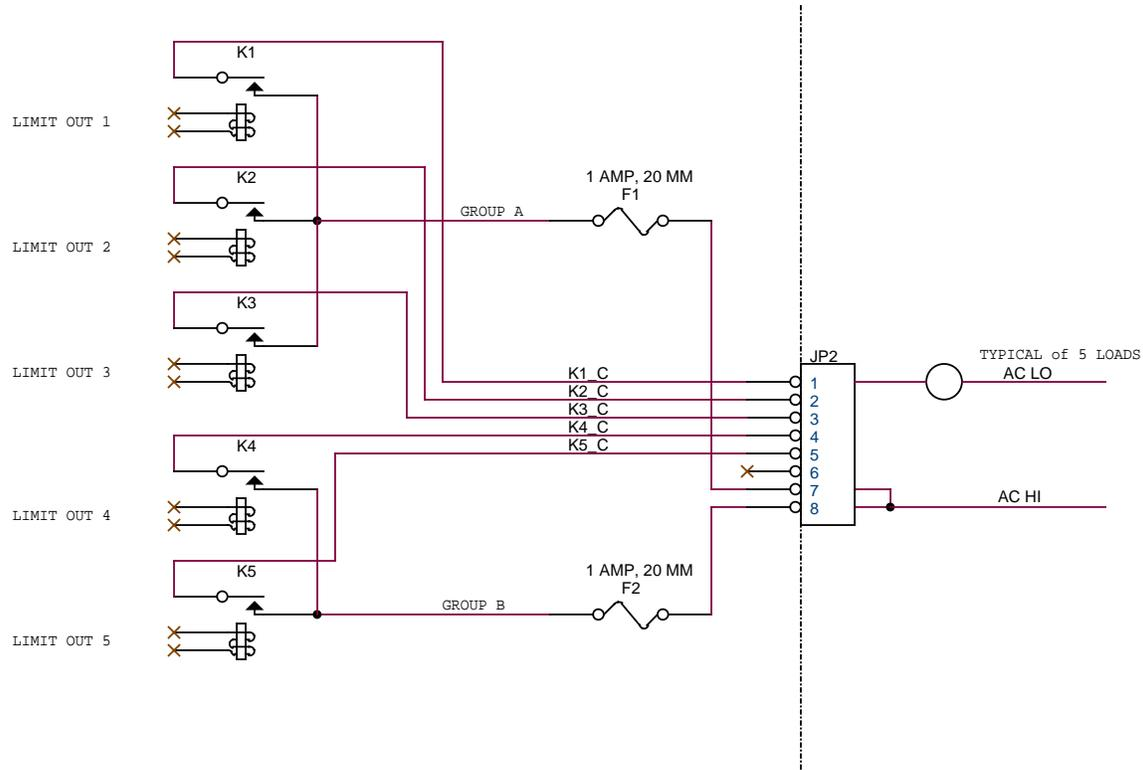
Figure 4 - Example Relay Limit Switch Connections
