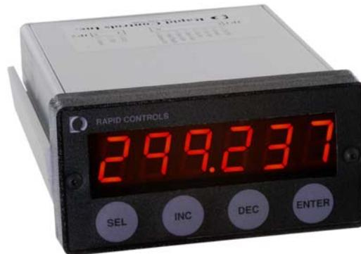
The TDD displays position information from a magnetostrictive transducer or quadrature encoder. It is capable of interfacing to a SSI, PWM, start/stop or neuter transducer depending on model. Setup is accomplished via the front-panel keypad or RS-232/485 serial communications link. The unit has optional programmable limit switches and analog output. A host computer can obtain position and limit-switch information via the RS232/RS485 serial link.
