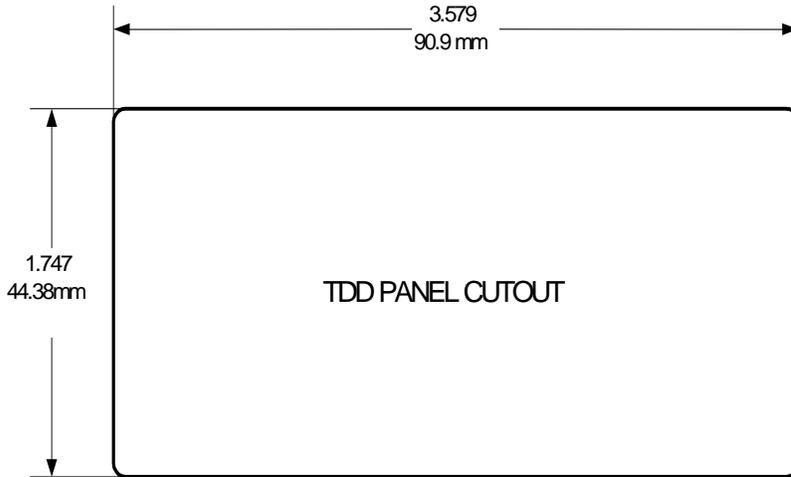
The TDD mounts into a panel and requires an 1/8 DIN panel space.
