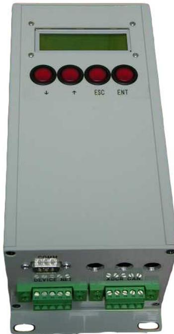
The XG555 CANbus to DeviceNet Temposonics Gateway gathers position information from as many as four Temposonics CANBUS transducers, each with multiple magnets. This information is provided to a host over a DeviceNet interface. Setup information is stored on the local flash disk. The system is comprised of an embedded industrial computer, with a PC-104 stack providing hardware interfaces. The PC-104 stack includes the processor, a CANBUS interface, and a DeviceNet interface.
