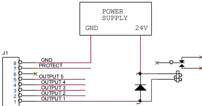
If you do not use the TDD internal kickback protection you must provide kickback suppression externally as above.
