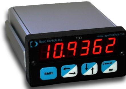
The TDD2 displays position information derived from a magnetostrictive transducer with Synchronous Serial Interface (SSI), Start/Stop, Pulse Width Modulated (PWM), or CANbus output. Setup of units, offsets, and other items can be accomplished via the front-panel keypad menu or a RS-232/485 interface.
