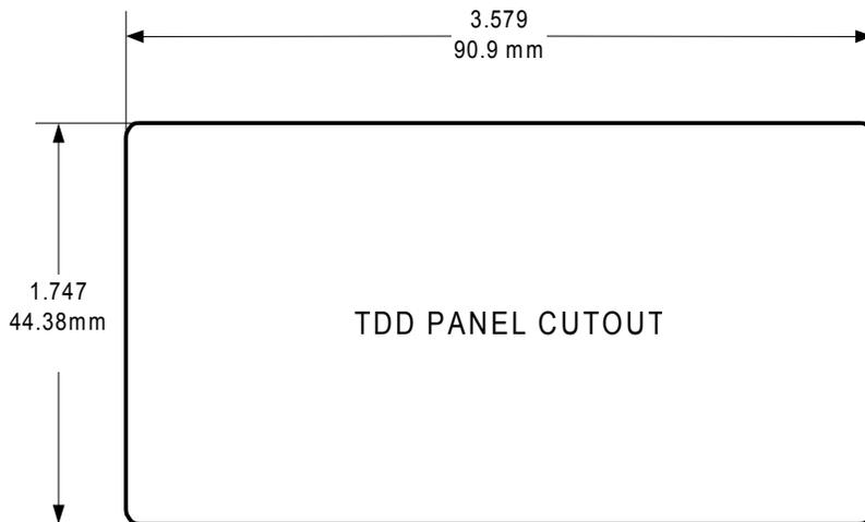
The TDD2 mounts into a panel and requires an 1/8 DIN panel space. It is approximately 5 inches deep from the panel including the connector.
